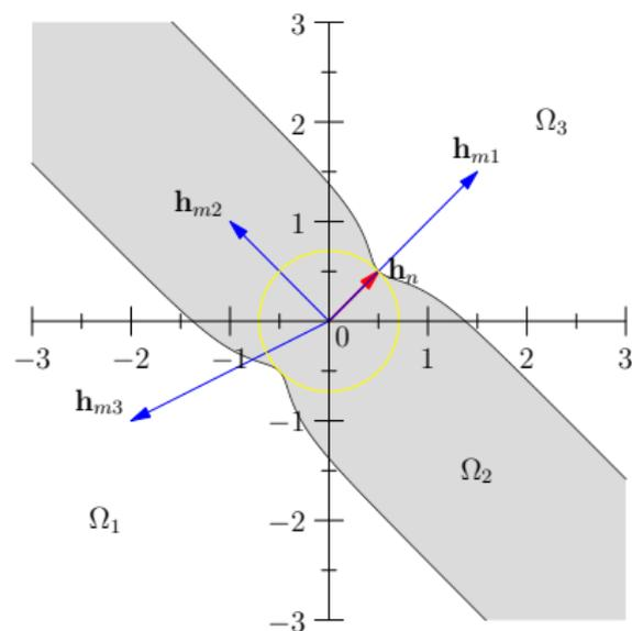
An illustration of quasi-degradation when a BS equipped with two antennas communicates with two single-antenna users.
