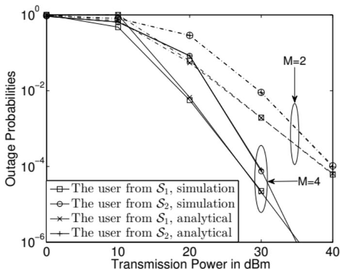
Outage probabilities achieved for Rayleigh fading channel model.  $|\mathcal{S}_1| = 1$ ,  $|\mathcal{S}_2| = M$ ,  $r_1 = 40\text{m}$ ,  $r_y = \frac{r_1}{2}$ ,  $\alpha = 3$ ,  $R_0 = 1$  BPCU and  $R_1 = 1$  BPCU.
