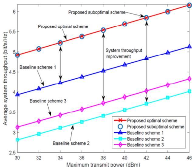
Average system throughput (bits/s/Hz) vs. the maximum transmit power at the BS (dBm),  $P_{max}$ , for different resource allocation schemes and 6 users.
