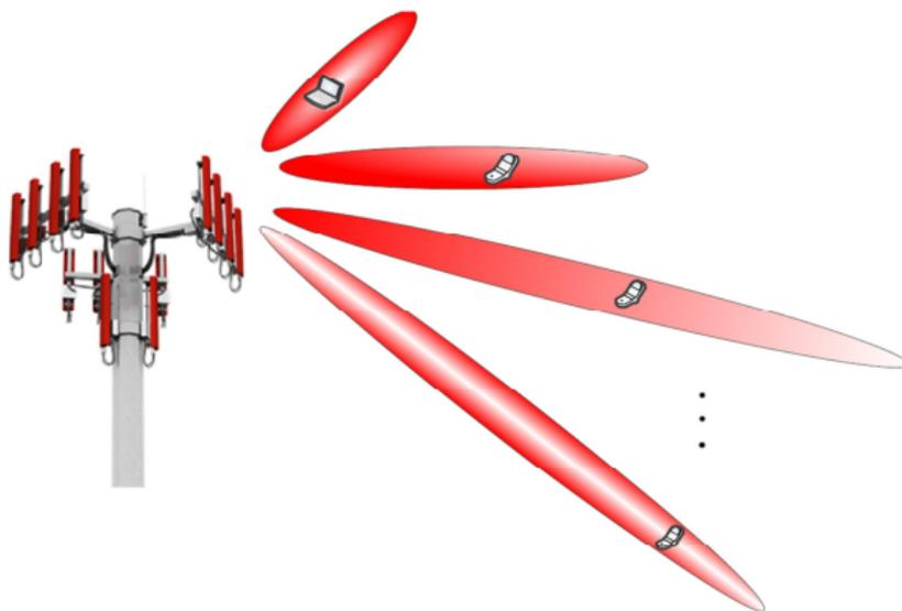
One type of MIMO-NOMA approaches is to assign users to beams individually and order users according to their path losses.
