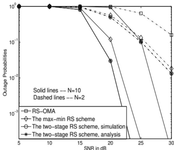
Comparison between cooperative OMA and NOMA with different relay selection (RS) strategies.  $R_1 = 0.5$  bit per channel use (BPCU),  $R_2 = 2$  BPCU, and  $\alpha_2 = \frac{1}{4}$ .
