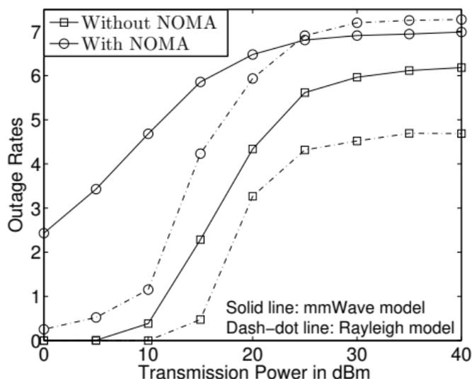
Outage rates achieved for different channel models.  $M = 30$ ,  $|S_1| = 3$ ,  $|S_2| = 300$ ,  $r_1 = 40\text{m}$ ,  $r_y = r_1$ ,  $\alpha = 3$ ,  $R_0 = 1$  BPCU and  $R_1 = 1.5$  BPCU.
